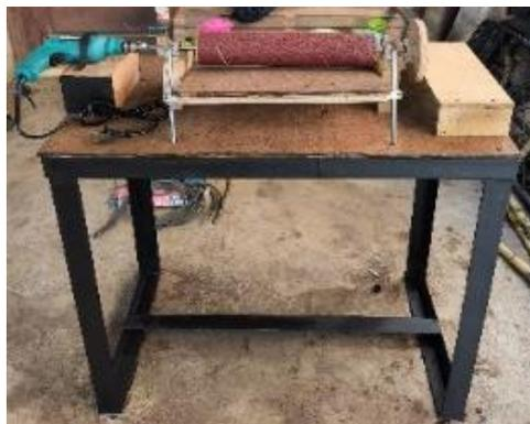
Gambar 2. Prototipe alat amplas 2 in 1
